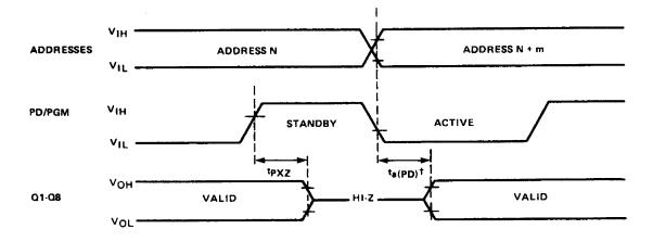
NOTE:  $\overline{\text{CS}}$  must be in low state during Active Mode, "Don't Care" otherwise.
